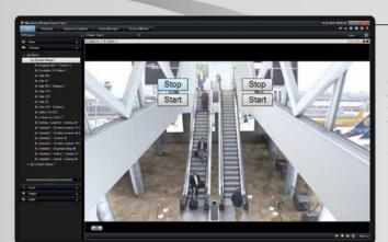
Integrated devices and other connected systems can be controlled directly with overlay buttons from the camera view, streamlining workflows and improving operator efficiency.
